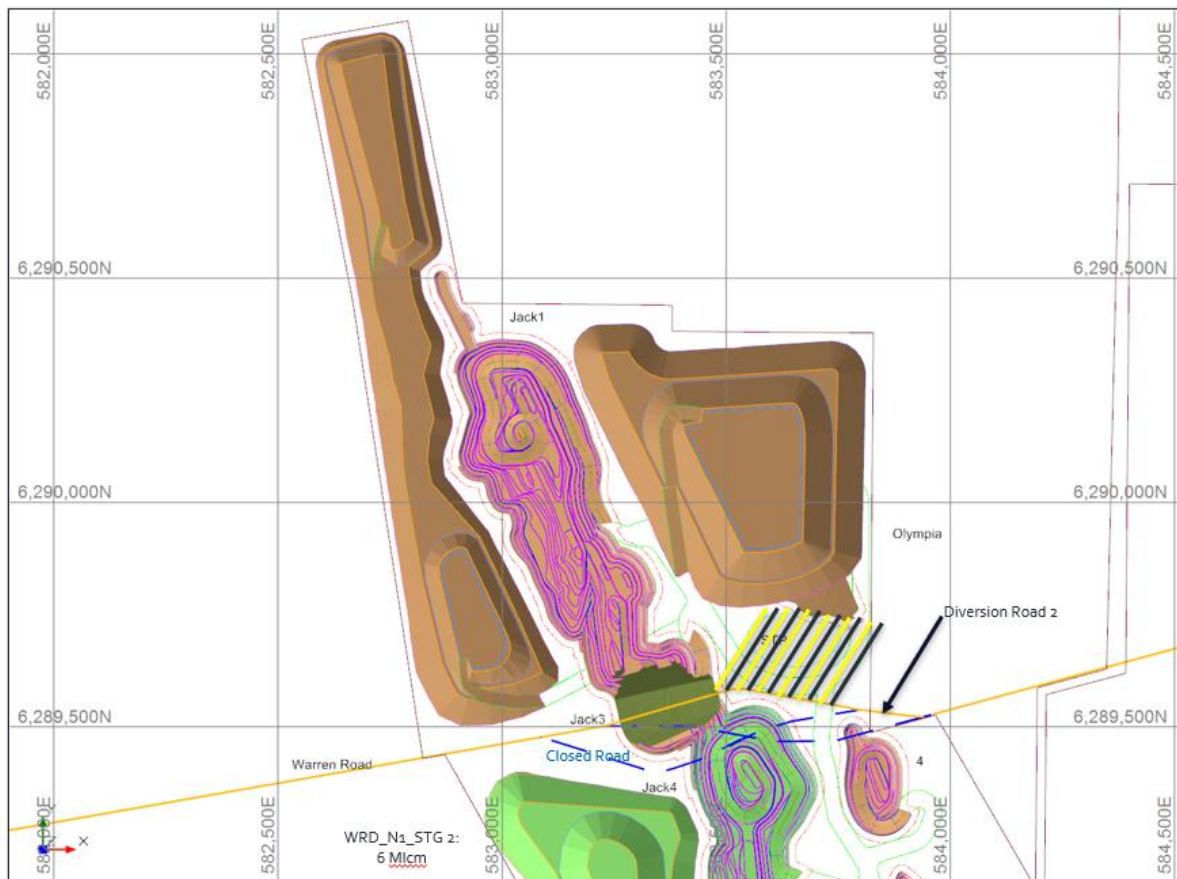
Figure 5-5: Northern Mining Area and Warren Road Solution
